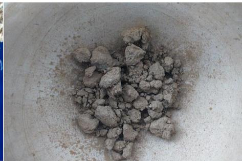
*Phot. 2. Roots mixed with soil clods ground with pestle in a mortar*
